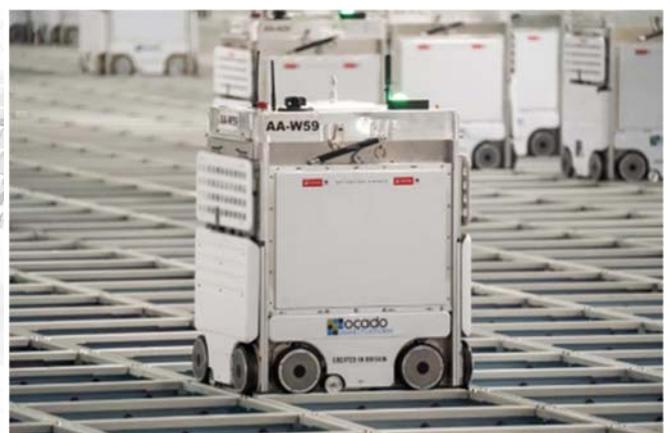
The CFC is characterized by its ability to hold a large range of approximately 50,000 products. It is enabled by 24 hours, highly efficient picking operations using robotics and AI. By utilizing Ocado's solution, the robots in the CFC can assemble a 50-item order within 6 minutes. Advanced AI algorithms are also used to constantly identify and update optimal routes for the most efficient home delivery.
